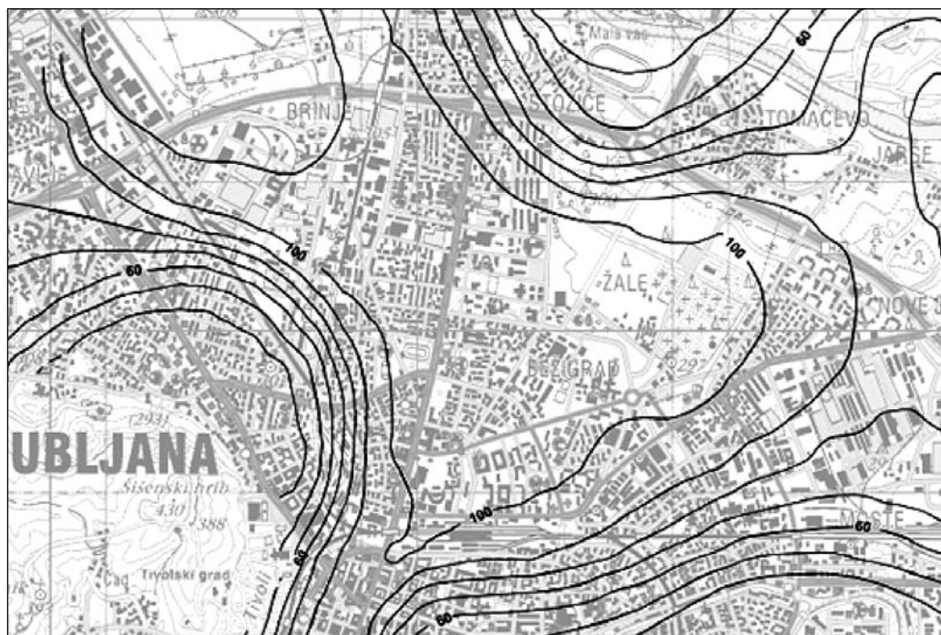
Figure 1: Contour lines of aquifer thickness on the Ljubljansko polje. North orientated.
